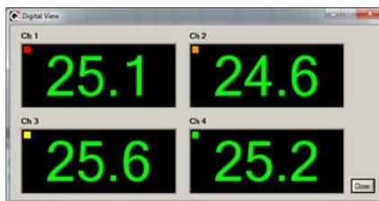
The size of this window will adapt to the number of channels to display. Up to 32 values can be shown. Refresh rate is always 1.0 sec.
