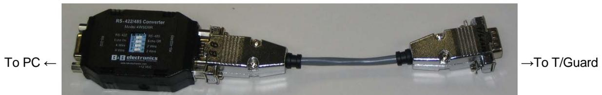
To use the converter, you will need a standard RS-232 cable that will attach your converter to your PC. Please note that PC's that do not have an RS-232 interface built-in will need an additional RS-232 to USB adapter that you can buy at any local computer shop<sup>21</sup>.
