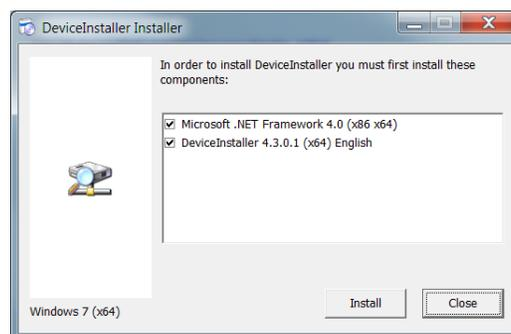
It is important that you install both the .NET and DeviceInstaller applications, as shown above. If you get a warning from your firewall, as shown below, you must click "Allow access".
